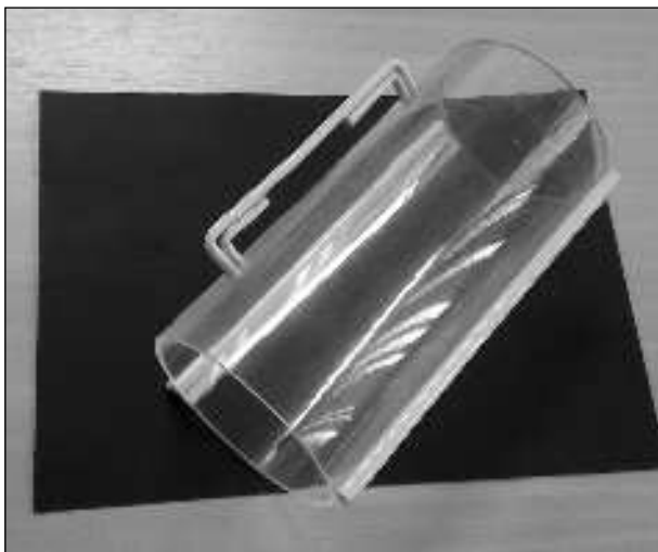
Figure 2. Acrylic cylinder of the phantom.
