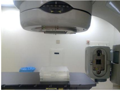
Fig. 1: Solid water phantom positioned on the irradiation table and gantry irradiation with output beam perpendicular to the phantom.
