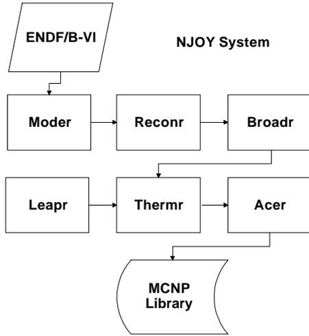
Figure 1. Cross Section Generation.
