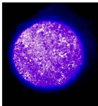
**FIGURE 3** - Fluorescent macroscopic image of PLGA  $[\text{Ru}(\text{bipy})_3]^{2+}$  nanosphers using blue light ( $\sim 450$  nm).
