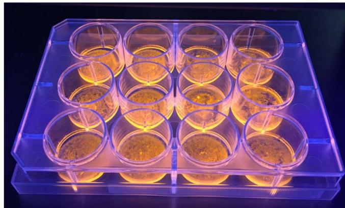
FIGURE 5 - PLGA [Ru(bipy)<sub>3</sub>]<sup>2+</sup> placed in 12 well-plate irradiate with blue light (~450 nm) ready to cells culture.
