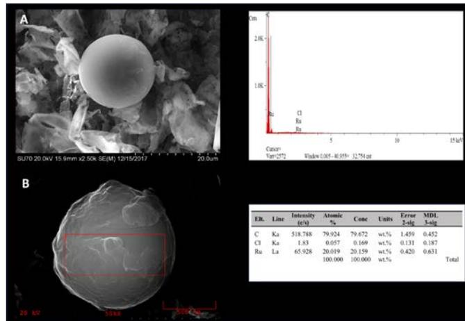
FIGURE 4 – SEM (20 kV) analysis (A) and Energy Dispersive X-Ray Analyzer (EDX) of PLGA [Ru(bipy)<sub>3</sub>]<sup>2+</sup> (B).
