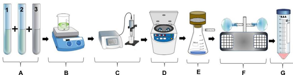
**FIGURE 1** – Sequence for  $\text{Ru}(\text{bipy})_3]^{2+}$  acetate-loaded nanospheres: (A) Mixture of PLG+PVA (1) with Ethyl Acetate (2) and 80Mn  $[\text{Ru}(\text{bipy})_3]^{2+}$  solution; stirring overnight (B); Solution was Sonicated (C) and centrifugation (D). After collected the supernatant it was washed, and filtration as made (E). Overnight lyophilizing was performed (F) to collect the NPRuBIPY (G).
