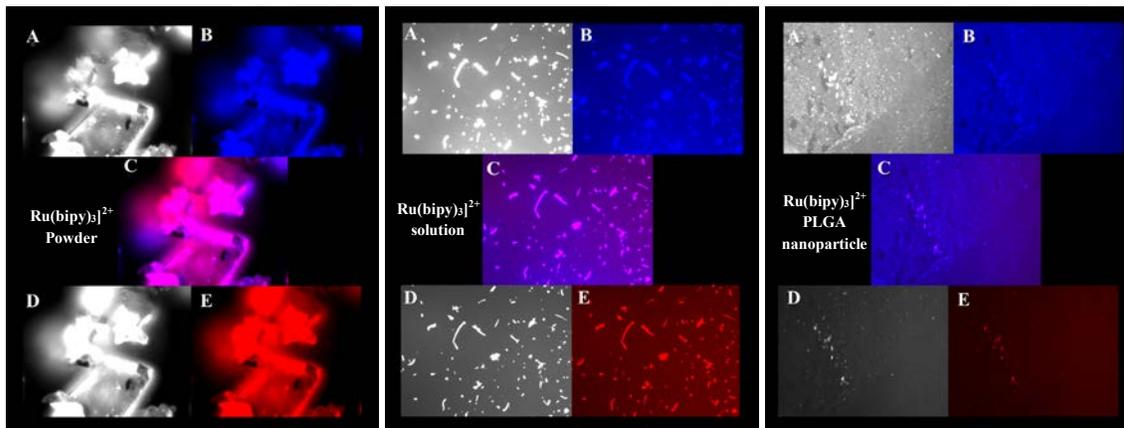
**FIGURE 2** - Fluorescent microscopic (100x) images of  $[\text{Ru}(\text{bipy})_3]^{2+}$  Powder (1);  $[\text{Ru}(\text{bipy})_3]^{2+}$  Solution (2) and PLGA  $[\text{RU}(\text{BIPY})_3]^{2+}$  nanosphers (3) at different intensities. Images 1 to 3 - A and D acquired in B&W raw; B excitation at blue light  $\sim 450$  nm; E excitation at red light  $\sim 620$  nm and C merged red and blue images (C).
