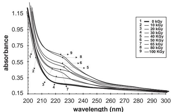
Fig. 1. Absorption spectra of Unipac-PE-60 samples before and after gamma irradiation doses up to 100 kGy.
