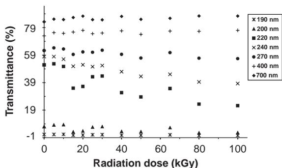
Fig. 2. Variation in % transmittance with radiation dose of Unipac-PE-60 samples after gamma irradiation doses up to 100 kGy.
