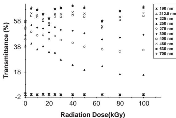
Fig. 4. Variation in % transmittance with radiation dose of Unipac-PA-30 samples after gamma irradiation doses up to 100 kGy.
