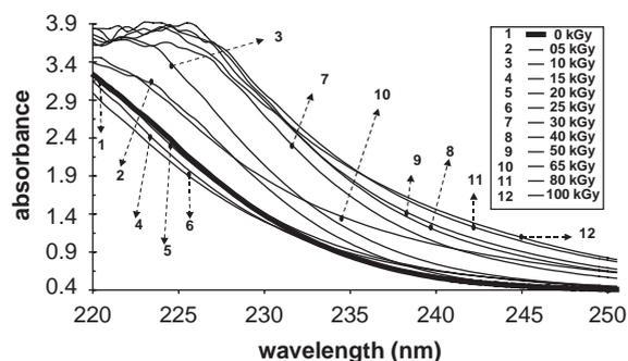
Fig. 3. Absorption spectra of Unipac-PA-30 samples before and after gamma irradiation doses up to 100 kGy.
