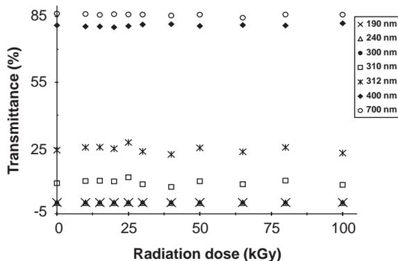
Fig. 5. Variation in % transmittance with radiation dose of Unipac-PET-12 samples after gamma irradiation doses up to 100 kGy.
