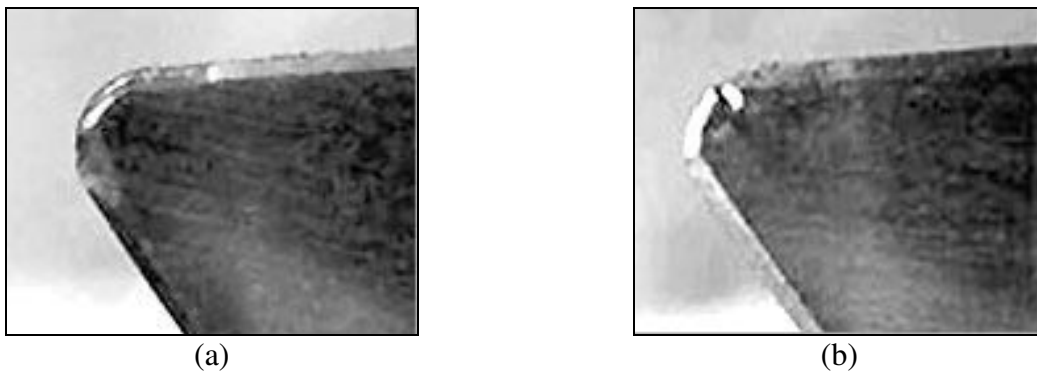
Fig. 7. Aspects of the ceramic tool surface submitted to flank wear. a) Ceramic tool aspect after machining the material under development (MD). b) Ceramic tool after machining the commercial material (CM).
