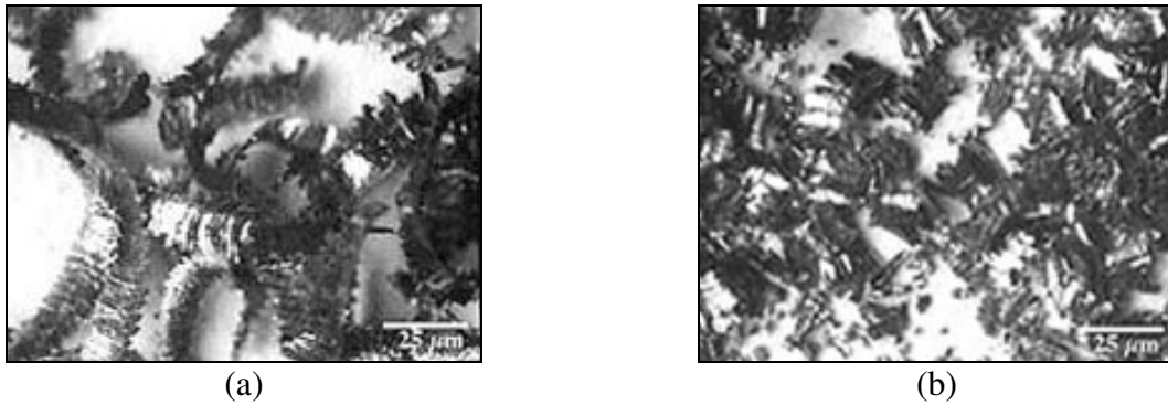
Fig. 8. Optical macrography of the machining chips. a) Connected arcs chips originated from the material under development (MD). b) Loose arcs chips originated from the commercial material (CM).
