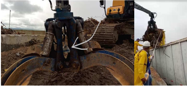
Figures 1 and 2 – Respectively, arrow indicating the packed detector, attached to the winch claw; and measurement made with rod.
