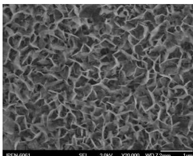
**Figure 1.** Scanning electron micrographs of HTC coating on AA 6061.
