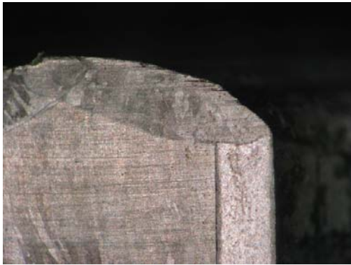
Figure 3 – Weld Joint Macrographic without indication of defects
