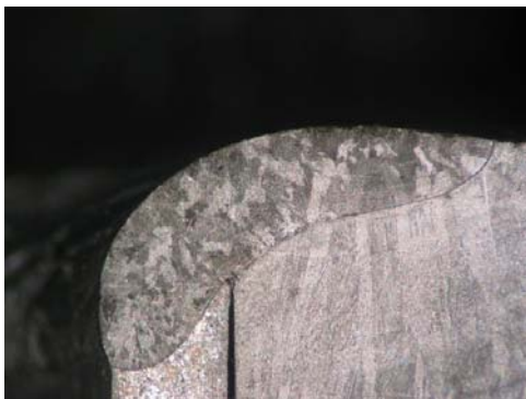
Figure 6 – Tube to tubesheet welding Macrographic “gap termination”
