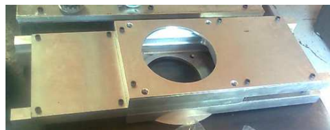
Figure 7. Attenuator device machined and partially assembled.
