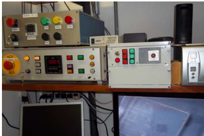
Figure 11. (a) Overview of the control modules of the radiators and the control panel of the attenuators exchange device; (b) Control panel of the attenuators exchange device of the OB85/1 Irradiator System.
