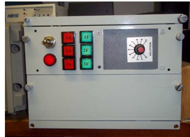
Figure 11. (a) Overview of the control modules of the radiators and the control panel of the attenuators exchange device; (b) Control panel of the attenuators exchange device of the OB85/1 Irradiator System.
