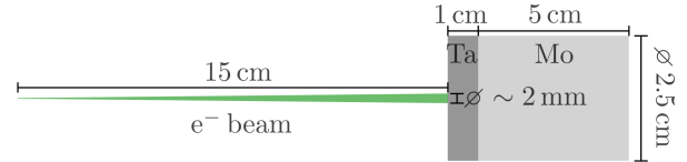
Fig. 1. Beam-target configuration (not to scale).
