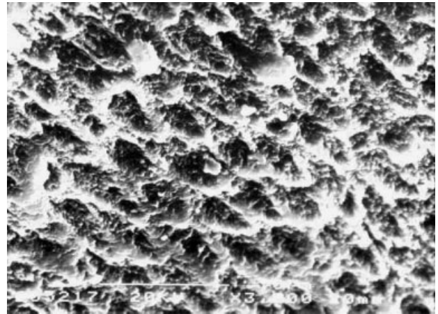
Figure 6 Scanning electron micrograph of sound bovine enamel after immersion in acetic acid. Treatment with 5% of acetic acid for 5 minutes in agitation
