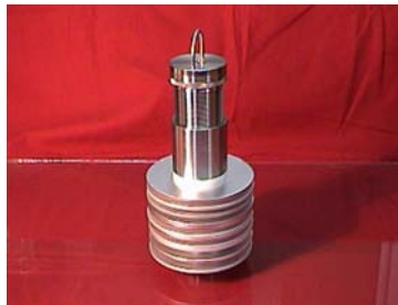
Figure 1. A typical corrosion test rack with coupons.
