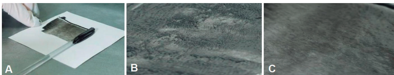
Figure 2 – Simple method recommended by the manufacturer: (A) Quality control procedure / (B) Example of poor quality dispersion / (C) Example of good quality dispersion (source: TUBALL™ MATRIX 300 series Processing Guide)
