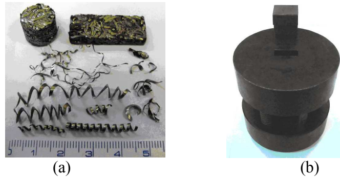
Figure 2 - Zirconium machining chips after cleaning and compaction (a). Rectangular press die (b).
