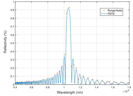
Fig. 3. Comparison between 4th-order-Runge-Kutta method and FDTD method. The red points represent the Runge-Kutta solution and the blue line represents the FDTD solution to 30 gratings.
