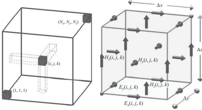
Fig. 1. A three-dimensional FDTD computational space composed of  $(N_x \times N_y \times N_z)$ .
