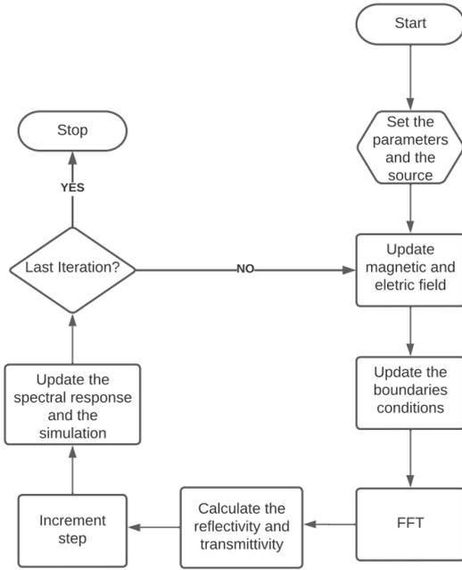
Fig. 2. Flowchart of FDTD algorithm implementation.
