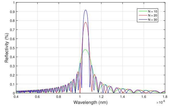
Fig. 4. Variation of the reflectivity coefficient for three different values of number of periods. It is possible to see that the greater is the gratings number, the stronger is the reflectivity.
