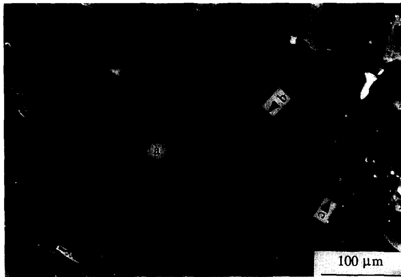
Fig. 1. Secondary electron image (tilt = 0°) of a polished cast Nd 15 Fe 77 B 8 sample on a JEOL 840A SEM. (a) matrix phase, (b) Nd-rich phase and (c) boron-rich phase.
