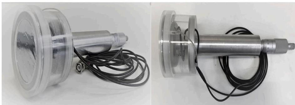
**Fig. 1.** Homemade extrapolation chamber developed at LCI/IPEN. Reproduced from Castro et al. (2020).
