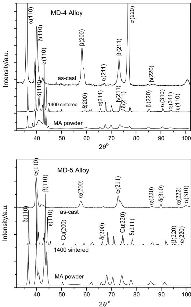
**Fig. 4** XRD profiles of MD-4 and MD-5 for as-cast, powder and sintered conditions
