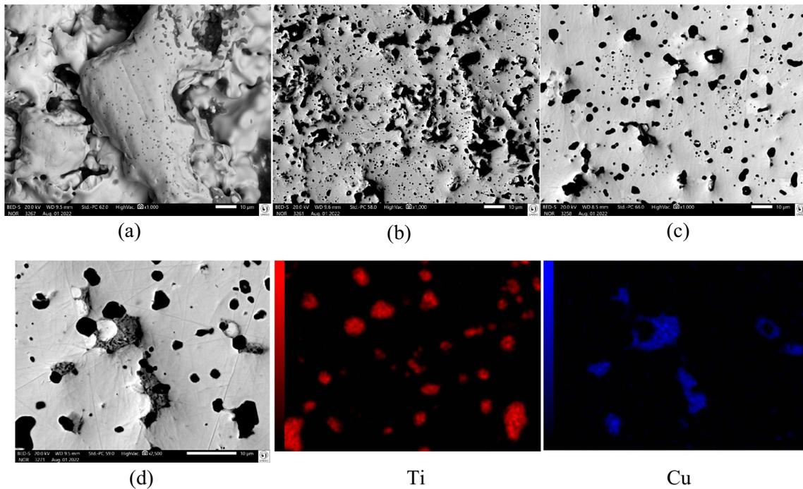
**Fig. 3** SEM images of 1500 °C sintered powder: **a** MD-4; **b** MD-5; **c** MD-5 + 3% Cu and **d** MD-5 + 3% Cu with corresponding Ti and Cu EDS maps
