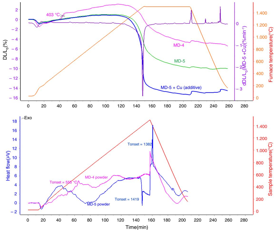
**Fig. 2** Dilatometric profiles up to 1500 °C under Ar-10%H<sub>2</sub>; pellets from powdered MD-4 alloy and MD-5 alloy with and without 3% Cu additive; retraction rate is also shown for MD-5 + Cu; below: DSC curves for MD-4 and 5 powders
