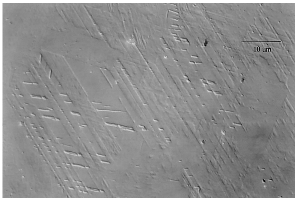
Fig. 3. Optical micrography of sample trained at 873 K showing \alpha' martensite (rod shaped).
