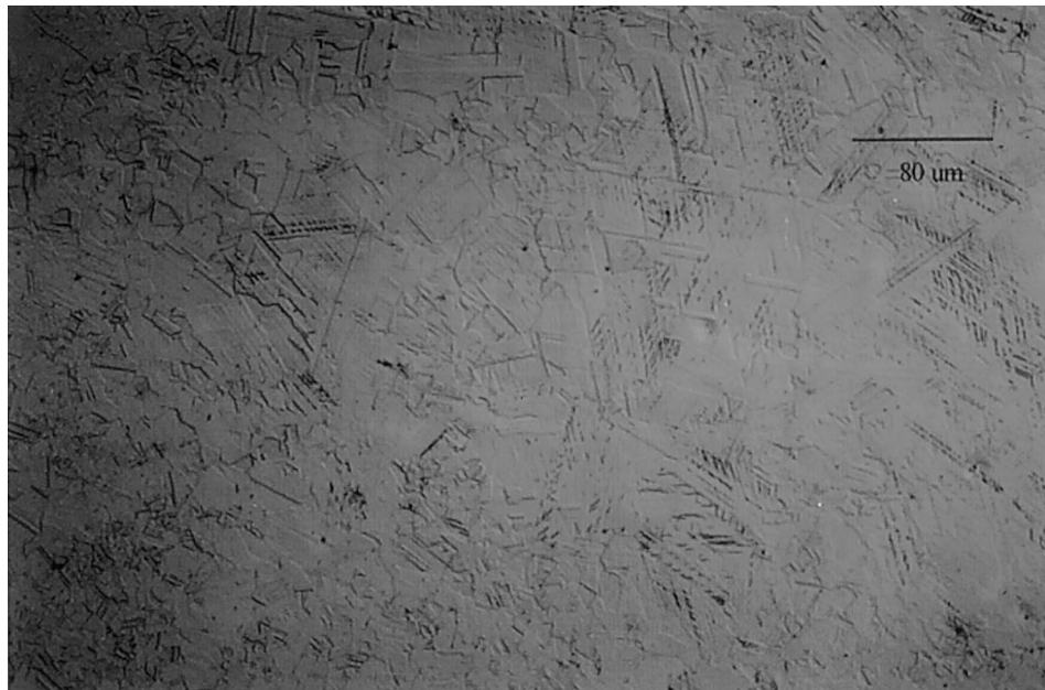
Fig. 4. Optical micrograph of the samples trained at 723 K showing precipitation of \alpha' martensite on large grains
