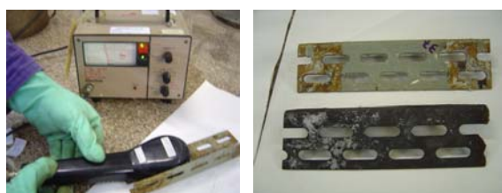
Figure 15: Monitoring (left), items before (above right) and after stripping (below right).
