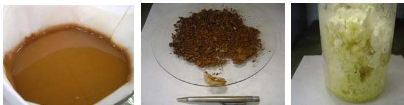
Figure 17: Salt solution filtration (left), radioactive waste, (center) and recovered salt (right).
