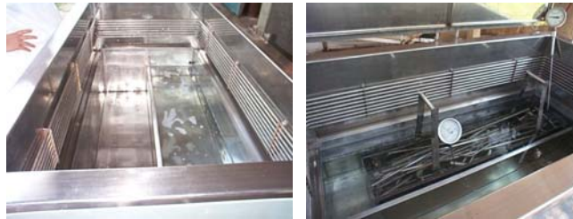
Figure 8: Internal view of the ultrasonic equipment and basket with contaminated parts.
