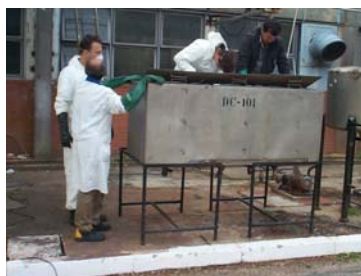
Figure 5: Stainless steel tank adapted for decontamination of components by pickling.
