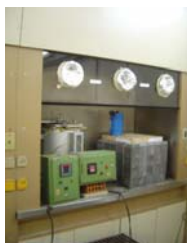
Figure 13: Molten salt stripping - exploratory system inside an exhaust chamber.
