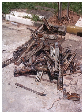
Figure 3: Perforated carbon steel structures after dismantling.
