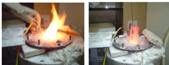
Figure 14: Molten salt stripping - introduction (left) and removal (right) of the sample.
