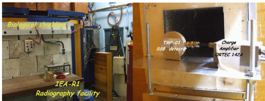
Figure 3: Neutronography assembly (left) and the TMF-01 detector setup (right)
