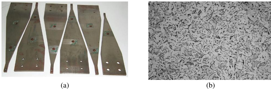
Figure 1. Instrumented constant stress cantilever beam (a) and microstructure of the ASTM A 36 steel plate used in the experiment.
