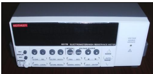
Fig. 2. Electrometer from Keithley Instruments Inc., model 6517B, used in this work in the characterization tests of the Böhm extrapolation chamber.
