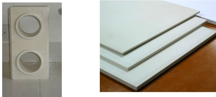
Figure 16: Bricks and plates made of phosphogypsum
