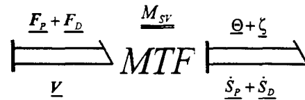
Fig. 6. Power coupling between the velocity and entropy ports.
