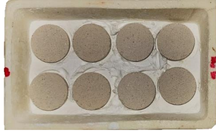
Figure 1: Pellets of glass and zeolite before sintering: V2ZAC_Sr; V4ZAC_Sr; V6ZAC_Sr; V8ZAC_Sr, from right to left.
