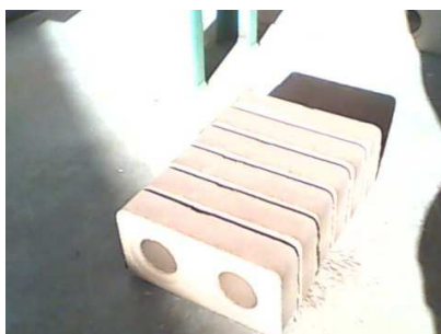
Fig. 1. Sludge from water treatment plant -coal fly ash-soil-cement bricks "Reprinted from ref. [22] with permission by the author"
