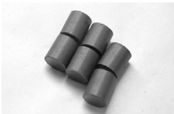
FIG. 21. Typical visual cracks on sintered pellets.
