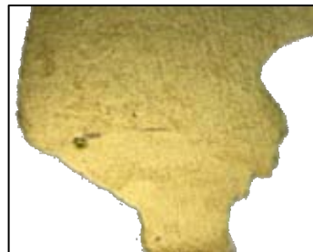
FIG. 28. Serious oxidation film
