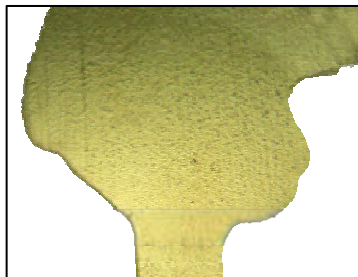
FIG. 27. Slight oxidation film
