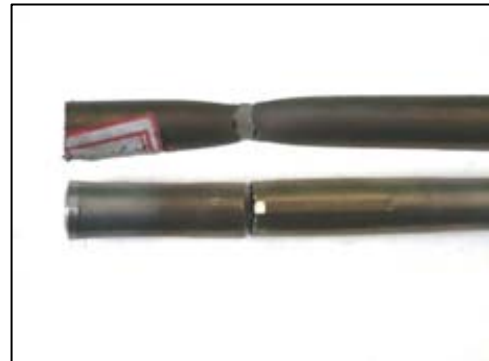
FIG. 6. Tensile test samples
