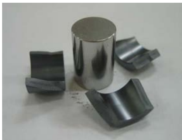
FIG. 8. Fractured annular pellet after tungsten rod inserted sintering.
