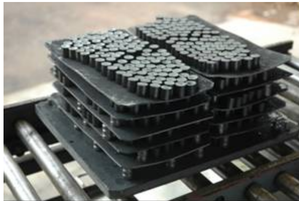
FIG. 4. Typical pellet loading pattern in a boat.
