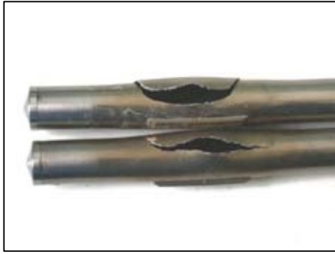
FIG. 7. Burst test sample
