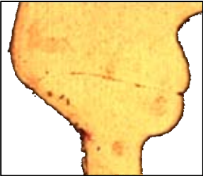
FIG. 12. Discontinuous welding lines in the welding joint
