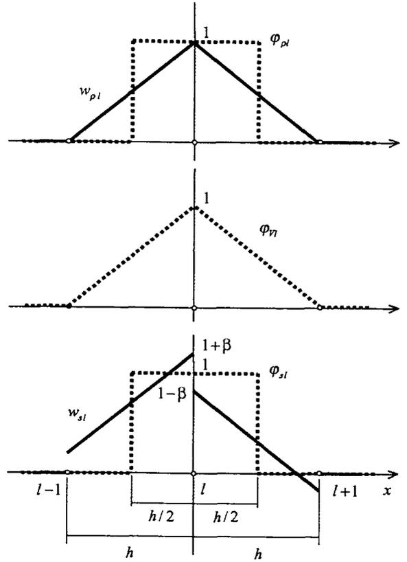
Fig. 2. Shape and weight functions
