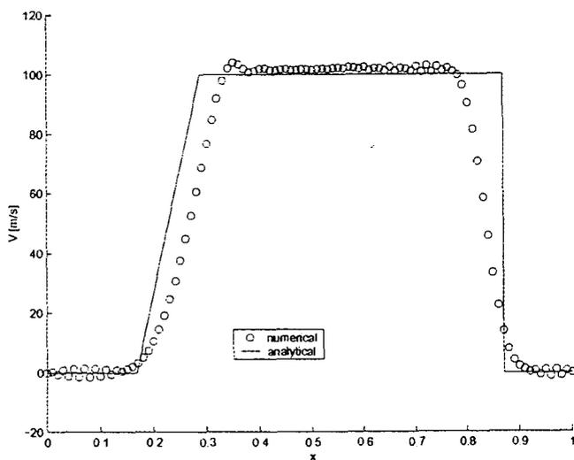
Fig. 6. Fluid velocity at  $t = 0.001$  s.
