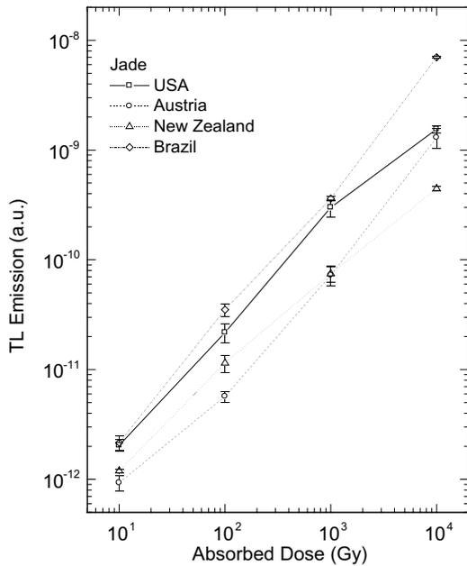
Fig. 6. Calibration curves of sintered jade pellets (<sup>60</sup>Co).
