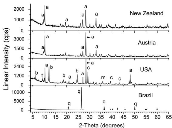
Fig. 1. Results of the X-ray diffractometry of the mineral samples acquired as jade. The symbols a, b, c, m, t and q means, respectively, actinolite, clinocllore, calcite, magnesiohornblende, talc and quartz.
