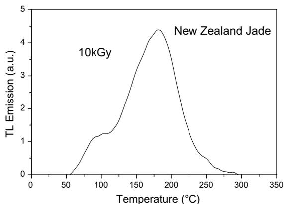
Fig. 4. TL glow curve of a sintered pellet of New Zealand jade irradiated with 10 kGy ( $^{60}\text{Co}$ ).
