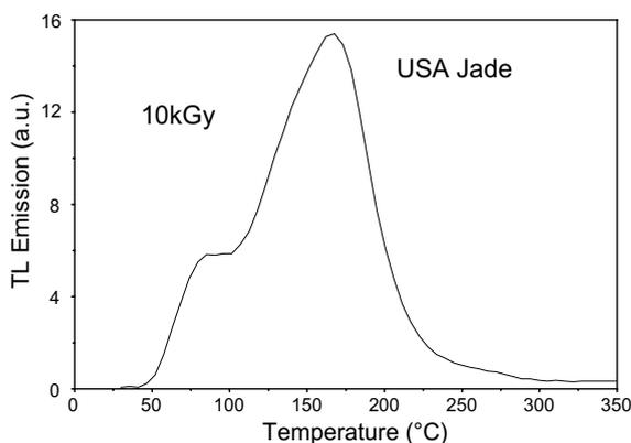
Fig. 2. TL glow curve of a sintered pellet of USA jade irradiated with 10 kGy ( $^{60}\text{Co}$ ).
