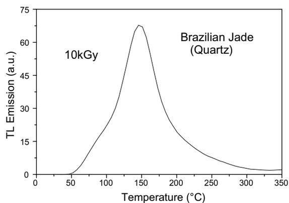
Fig. 5. TL glow curve of a sintered pellet of Brazilian jade irradiated with 10 kGy ( $^{60}\text{Co}$ ).
