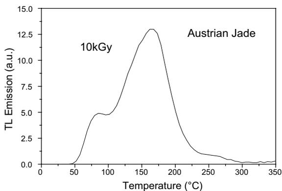
Fig. 3. TL glow curve of a sintered pellet of Austrian jade irradiated with 10 kGy ( $^{60}\text{Co}$ ).
