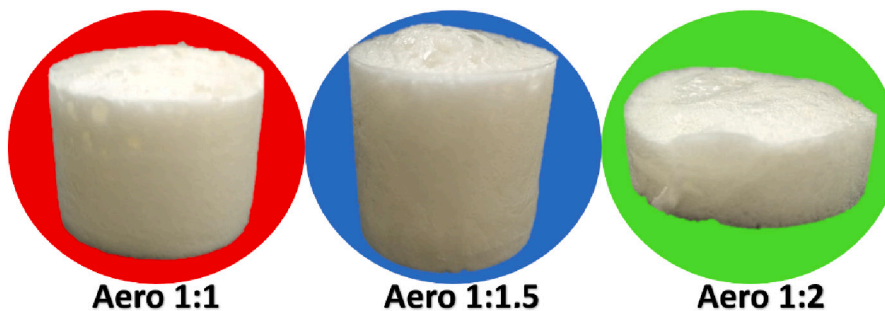
Fig. 3. The visual aspect of corn starch aerogels, highlighting Aero 1:1 (red circle), Aero 1:1.5 (blue circle), and Aero 1:2 (green circle), respectively.
