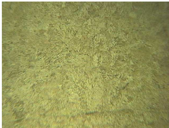
Figure 10: Typical micrograph of the cardan yoke tempered by induction.
