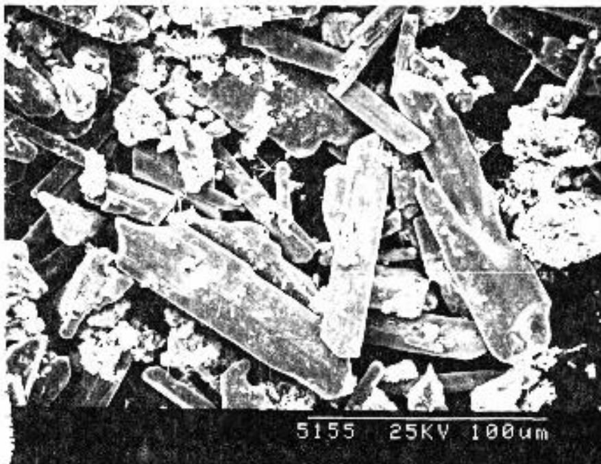
Fig. 4.8. SEM micrographs of 211 particles extracted from quenched semisolid mixtures formed by incongruent melting of type B 123 samples. Sample held at 1094°C, in air, for 30 min, and then quenched in water. Particles extracted by ultrasonically the quenched sample in de-ionized water for 1 h. The 211 particles were also faceted, but more irregular than the type A particles. Hollow and branched particles were commonly observed in these samples.
