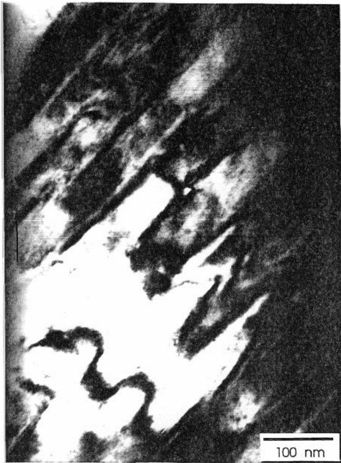
Fig. 5.29. Twins in a single-grained orthorhombic LHFZ filament (Sample 029). The plane of the TEM foil was parallel to the filament axis. The twins are observed at a 45^\circ angle to the growth direction (arrow), suggesting that the growth direction was [100].
