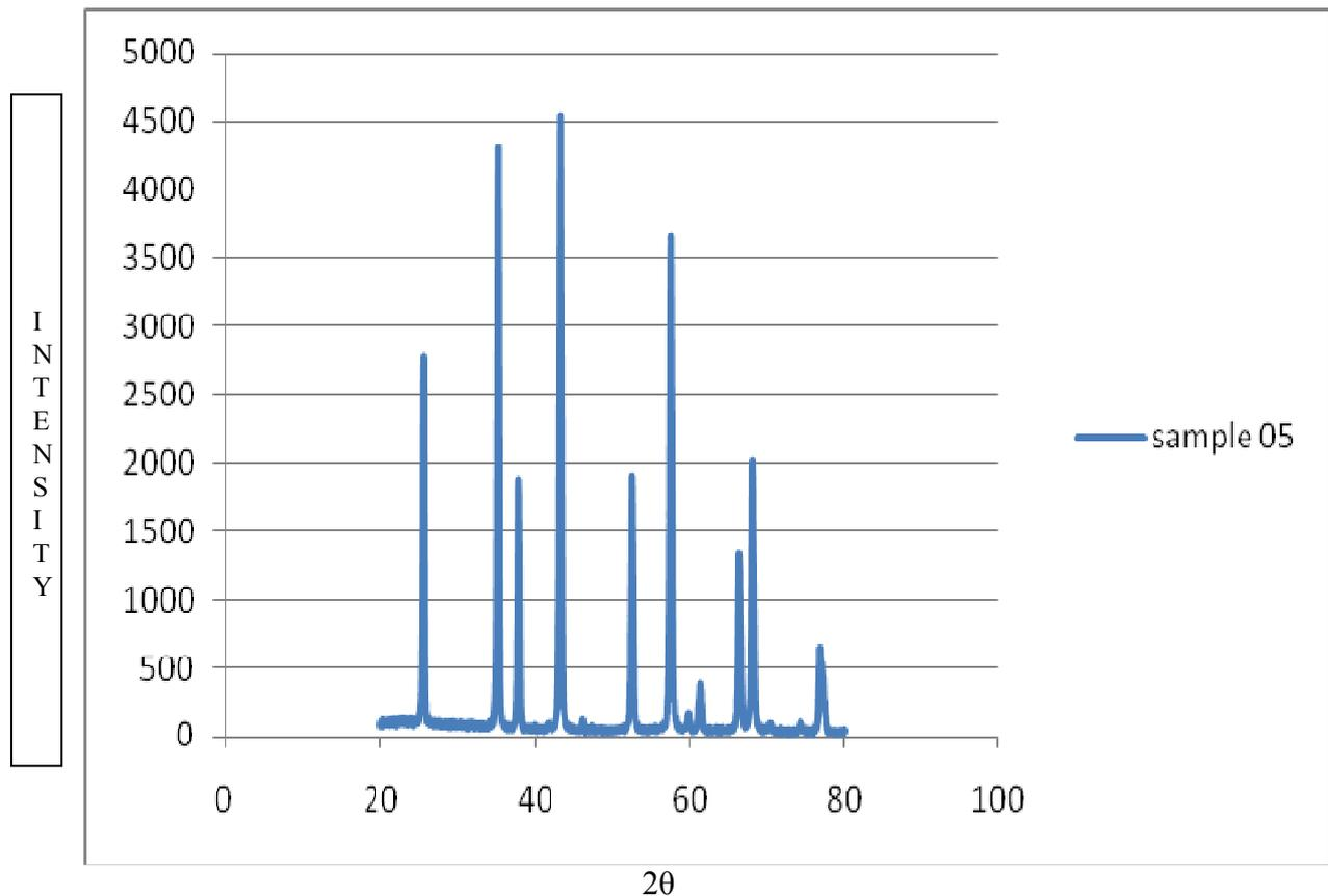
Figure 3 X-ray diffraction data of sample 5.
