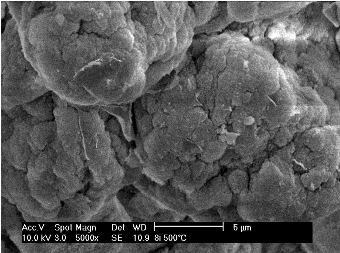
Figure 2. Micrograph of sample 16 calcined at 500° C: magnification of 5000X
