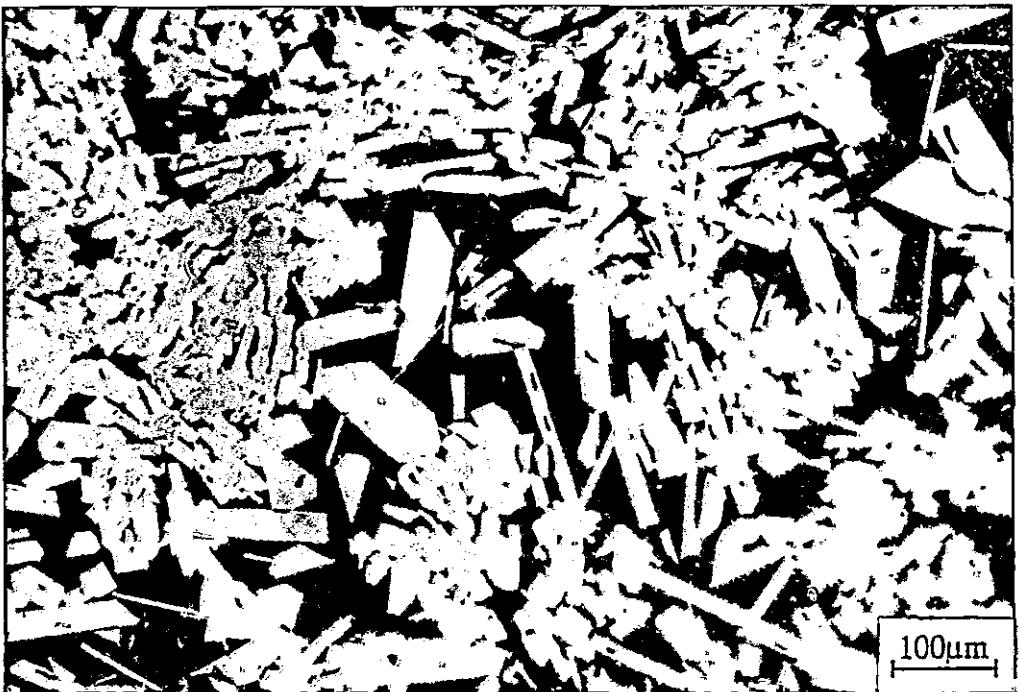
Fig 8.6.4 Microstructure of VFZ annealed alloy II( 63.5 cm/h ).
