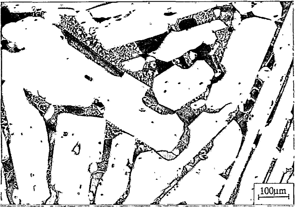
Fig 8.6.3 Microstructure of VFZ annealed alloy II( 25.4 cm/h ).
