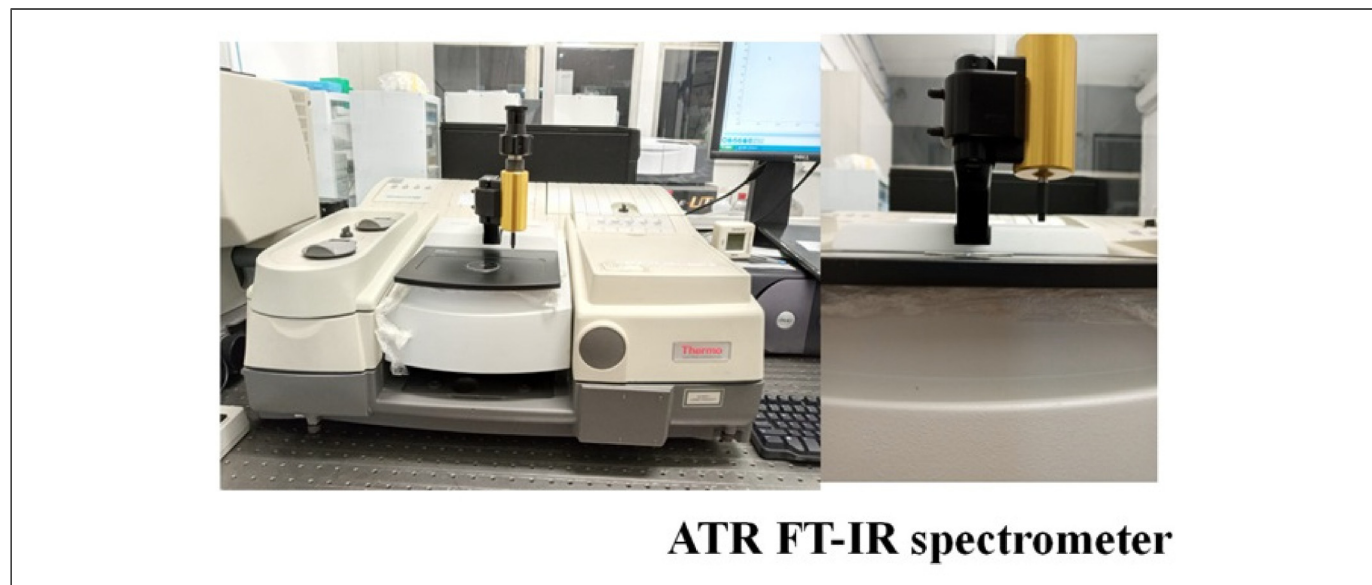
Figure 1. Shows the equipment and the crystal where the sample is dried.
