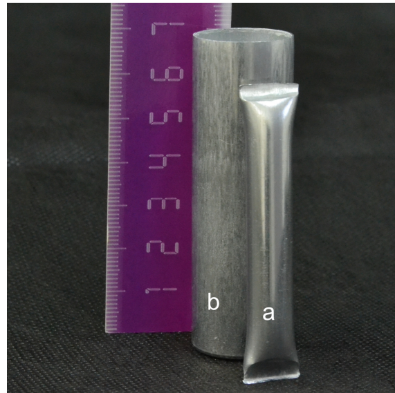
Figure 1: (a) Aluminum capsule to irradiate gaseous samples and (b) standard aluminum rabbit used to irradiate solid samples in nuclear reactor IEA-R.
