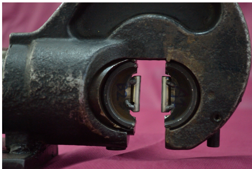
Figure 2: Hydraulic presshead with semi-circular slotted die modified.
