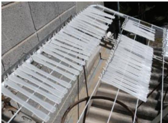
**FIGURE 1.** Device with dumbbell samples exposed outside for environmental ageing at the polymer processing laboratory IPEN.
