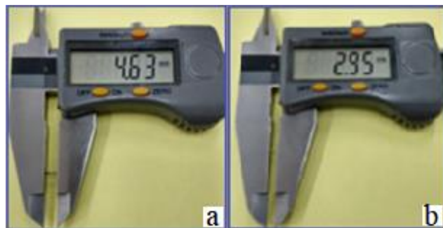
Figure 2. (a) Physical measurement of the length of the iodine-125 seed, (b) measurement of the core.
