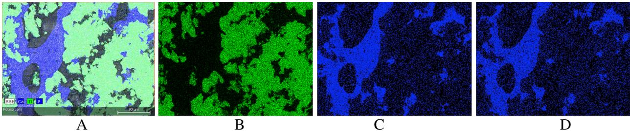
Figure 1. Example of SEM-EDS analysis of cpTi sample: A) Composite image highlighting Ti, Ca, and P all together; B) Image highlighting only Ti, green color; C) Image highlighting only Ca, blue color; D) Image highlighting only P, blue color.
