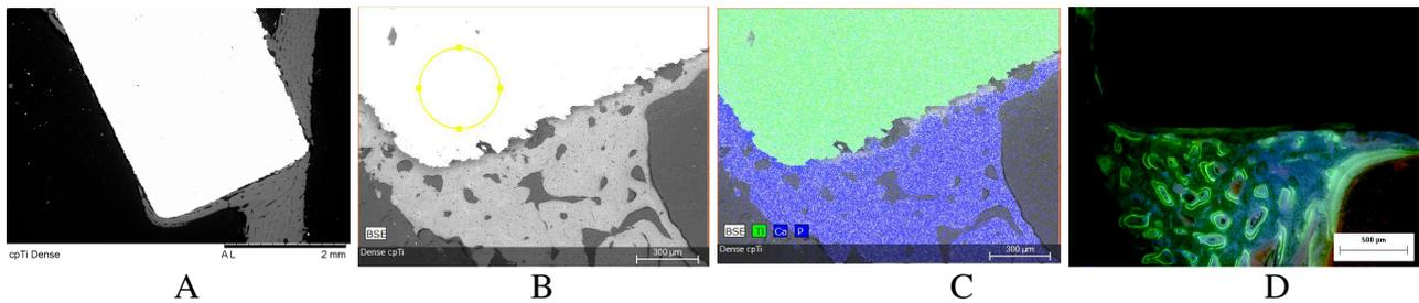
Figure 11. Machined dense cpTi Implant: A) SEM of histological slide, osteoconduction through the surface of implant; B) SEM of histological slide showing in detail the interface bone-implant; C) SEM-EDS of histological slide of image presented on B; D) FM analysis of bone markers, bone-implant interface.
