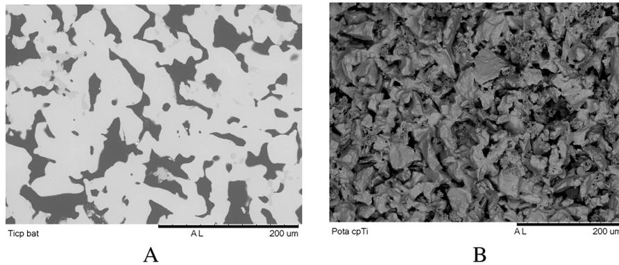
Figure 8. SEM of microstructure of the samples added potato starch: A) polished, B) fractured.
