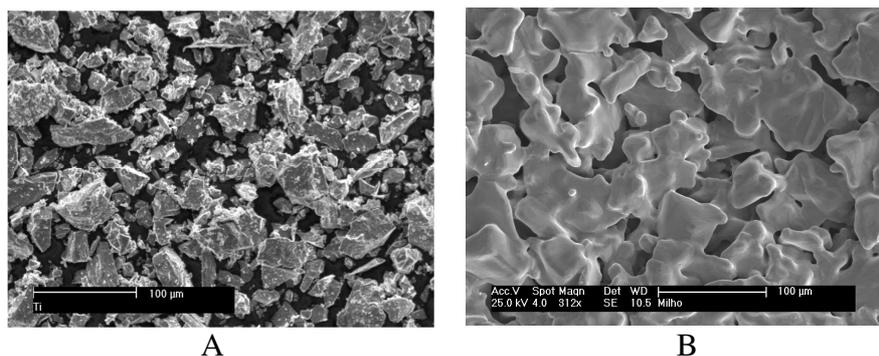
Figure 3. SEM. A) TiH<sub>2</sub> powder morphology [25]. B) Example of surface morphology after sintering.
