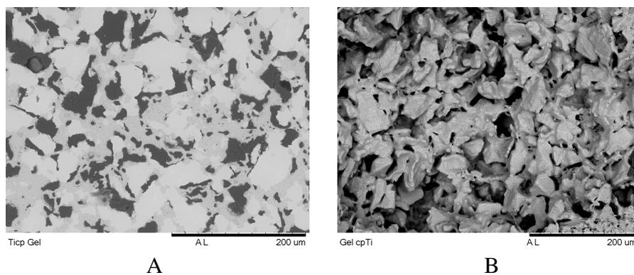
Figure 10. SEM of microstructure of the samples added gelatin: A) polished, B) fractured.
