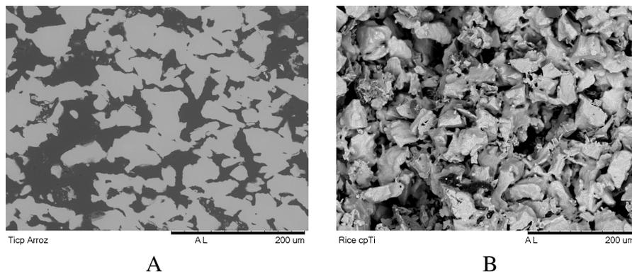
Figure 9. SEM of microstructure of the samples added rice starch: A) polished, B) fractured.
