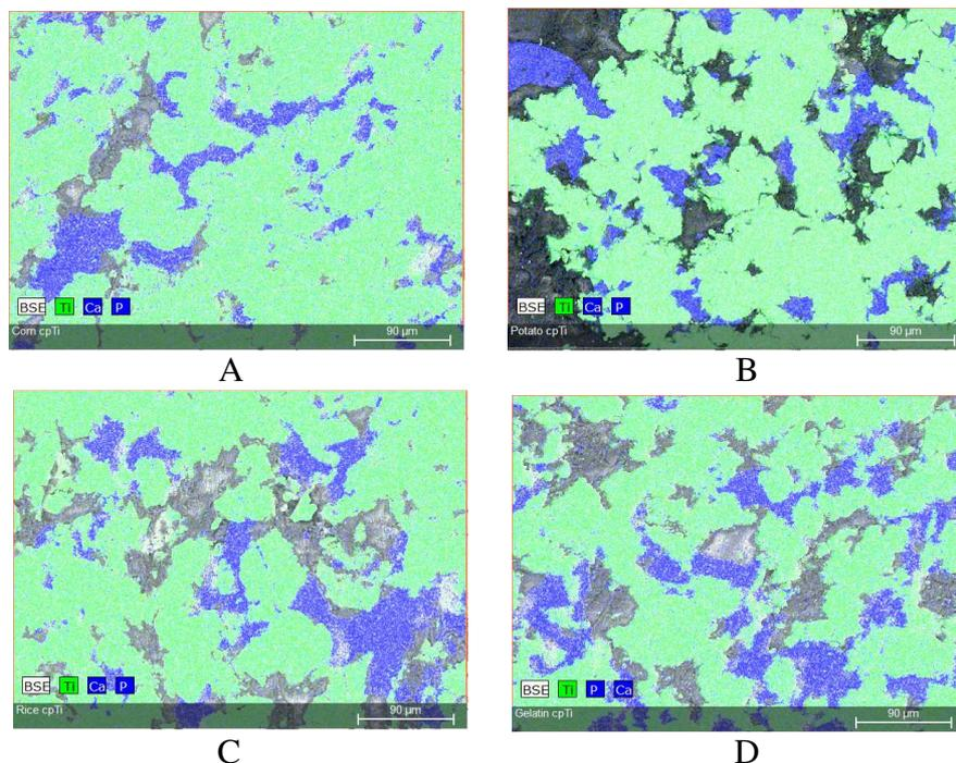
Figure 14. SEM-EDS of histological slice, showing pores (grey), bone (blue) and implant (green) areas, of samples added: A) cornstarch, B) potato starch, C), rice starch, D) gelatin.
