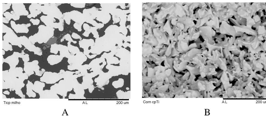
Figure 7. SEM of microstructure of the samples added cornstarch: A) polished, B) fractured.
