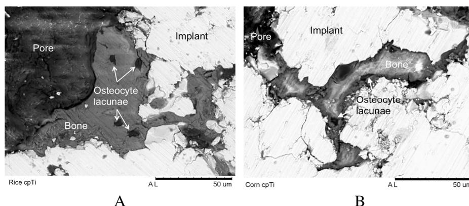
Figure 13. SEM of undecalcified histological slide presenting bone-implant interface and pores; osteocyte lacunae indicated by arrows: A) Implant obtained with rice starch, B) Implant obtained with cornstarch.
