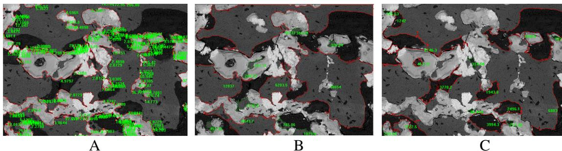
Figure 2. Example of image analysis of the bone-implant elements, delimited by red line: A) Implant area, represented by light grey, white color; B) Bone area, represented by dark grey color; C) Empty pores area, represented by black color.
