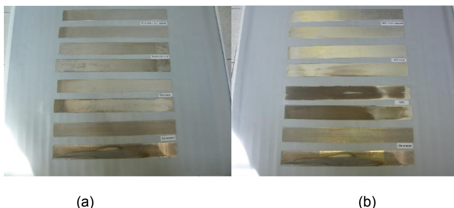
Fig 7: Photographs of full-size plate surfaces. (a) Boehmite coated and (b) HTC coated. The plates above the identification mark were exposed for 8 months and the plates below, for 14 months.
