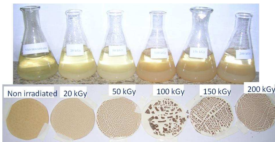
Figure 7. Precipitate of degraded cellulose from sugarcane bagasse after irradiation in various absorbed doses.
