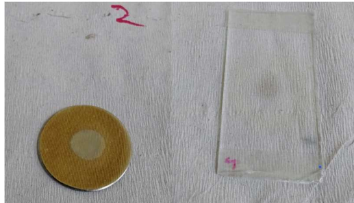
Figure 5: A representative photograph of an irradiated sample. The patterning promoted by the laser raster is visible on the sample, and the brownish spot at the center of the glass slide is also perceivable, indicating the metal deposition.
