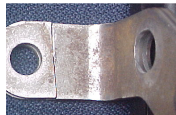
Figure 12: Support failure region.
