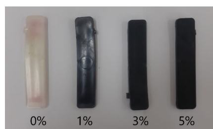
Figure 1. Izod specimens of HDPE/RHA composites, with 0, 1, 3, and 5 wt% of RHA filler.
