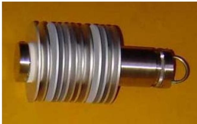
Figure 1. RLA project rack with coupons.
