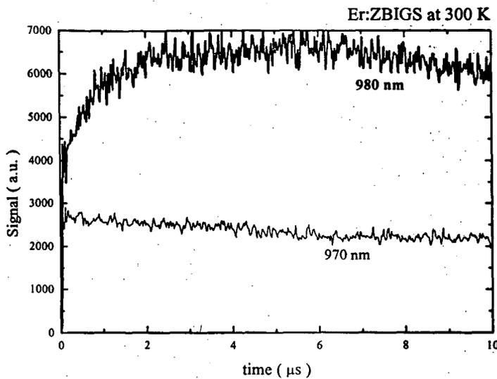
Figure 2 - Comparison between ESA (970 nm) and ETU (980 nm) rise times for the green emission.
