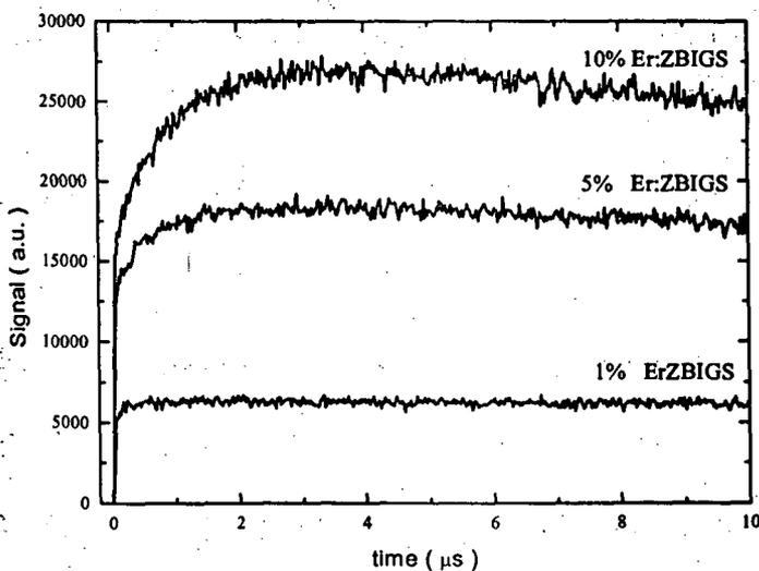
Figure 3 - Comparison between ESA and ETU rise times for the green emission at different Er concentrations. ESA is the main effect for small concentrations and ETU is more relevant for concentrations greater than 5 mol %.
