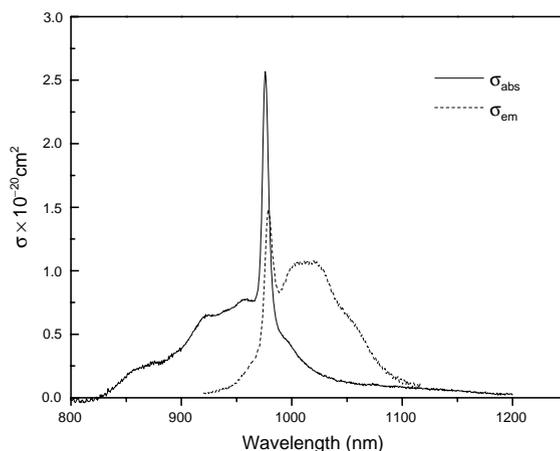
Fig. 1. Absorption and emission cross-sections spectra for the lead fluoroborate glass with 0.5 mol% of  $\text{Yb}_2\text{O}_3$ .
