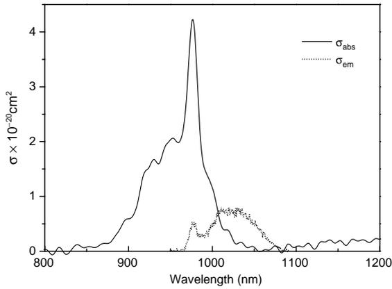
Fig. 3. Absorption and emission cross-sections spectra for the niobium tellurite glass with 5 mol% of  $\text{Yb}_2\text{O}_3$ .
