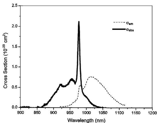
Fig. 2. Absorption and emission cross-sections spectra for the heavy metal oxide glass with 0.5 mol% of  $\text{Yb}_2\text{O}_3$ .
