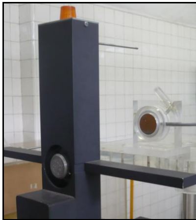
Fig. 1 Experimental set-up used in the measurements with the parallel plate ionization chamber and the ^{90}\text{Sr}+^{90}\text{Y} source (1850 MBq, 1981)
